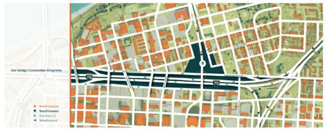
This option would maintain the current I-70 alignment. Highway 9 would be brought down to grade and connect at Independence Ave. and 6th Street. Independence Ave. would be reconnected across Highway 9 and maintain one-way (Westbound).
